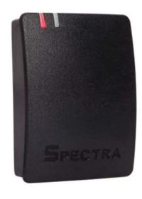
M20 Proximity reader is indigenously developed high performance reader to read Mifare read only cards. It provides a consistent read range of 4~5 cm in most of the conditions. The reader is particularly suited to access control applications. The same basic unit can be configured to most common output interface formats, including Wiegand, Magstripe and RS-232 serial ASCII.
